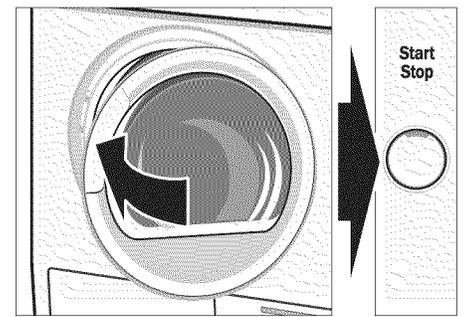
7. Press the **Start/Stop** button. The **Start/Stop** indicator light illuminates.
