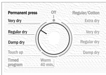
The program sequence of automatic programs is controlled via sensors. The duration of the program depends on the measured degree of moisture in the laundry and on the selected degree of dryness (e.g. damp dry or extra dry).
