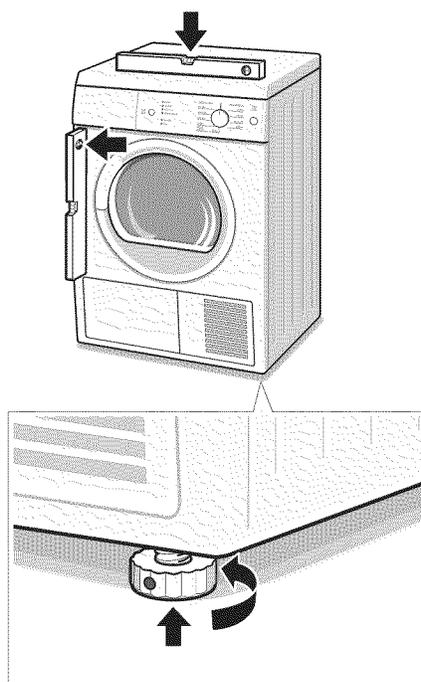
The dryer should be level with all four feet firmly on the ground. The dryer must not wobble.
