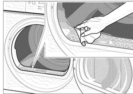
This deposit can easily be removed by wiping the sensors (the two bars next to the lint filter) with a cloth and a little white vinegar. Use white vinegar only! Clean the moisture sensor once a month.
