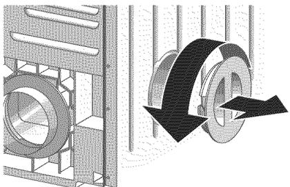
2. Remove the bayonet ring from the rear panel and attach it to the side panel vent.
