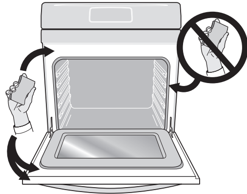
Figure 45: Oven door area to clean and not clean (gasket).
