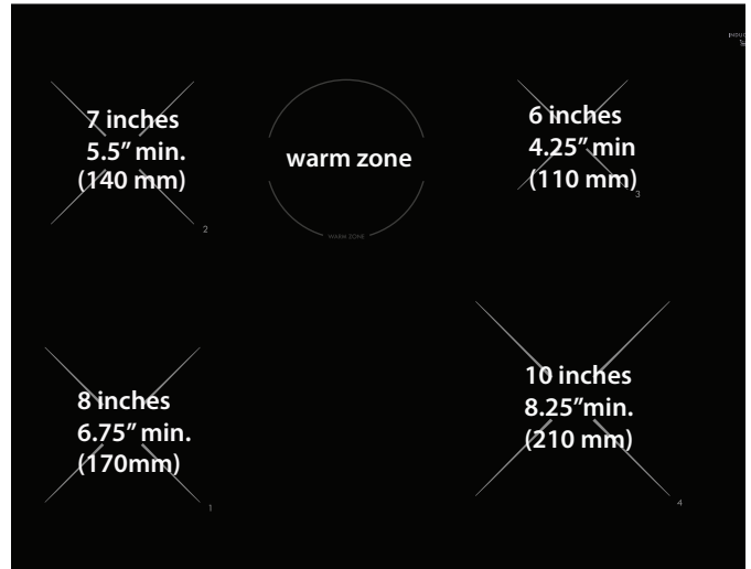
Figure 4: Induction cooking zone sizes
